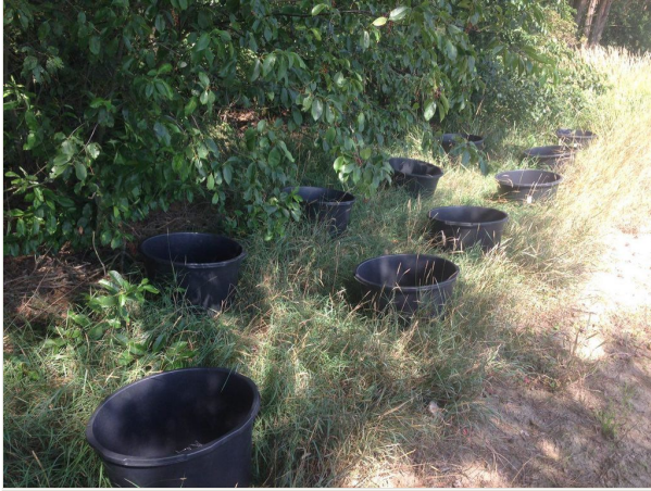
Figure 7. Setting of litter fall traps at the zero line (edge).
