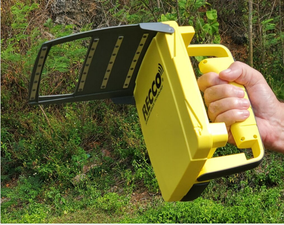
Figure 4. RECCO hand-held harmonic radar transceiver.
