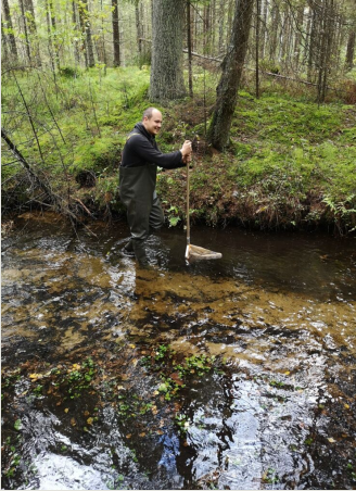
Figure 2. Sample collection using the Kick Sampling method by using D-shaped aquatic net.
